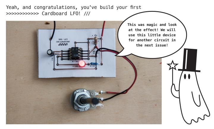
There are some things to say. The IC-Socket has to be placed first. The last component, which has to be placed on the board, is the 555 Timer IC. Make shure, that your parts will have the right polarity. If your LED won't light up, then you have to check your connections.
