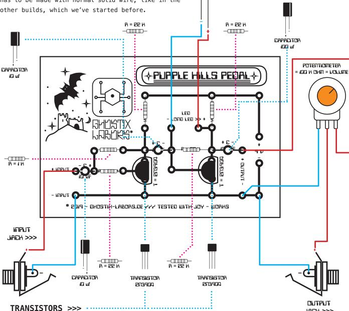
The orientation of the two transistors is directly shown on the surface of our board. The flat side faces to the right. If they are placed in the wrong direction, your project will not work.
